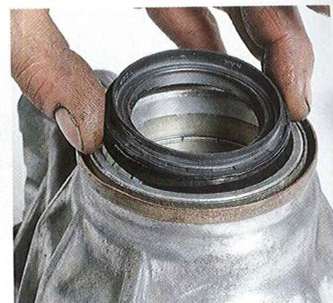
19 | Installer le joint spi neuf.
